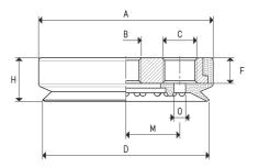
Note: The force of the vacuum cups indicated in the table represents 1/3 of the value of the theoretical force calculated at a level of vacuum of -75 KPa and a factor of safety 3. Transformation ratio: N (newton) = Kg x 9.81 (force of gravity) inch =  $\frac{mm}{25.4}$ ; pounds =  $\frac{g}{453.6}$  =  $\frac{Kg}{0.4536}$  Adapters for GAS - NPT threading available on page 1.130
