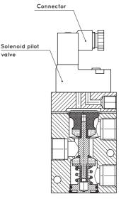
N O X = Compressed air supply P = Discharge A = Use R = Pump
