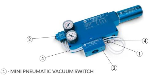
The vacuum switch has the task of removing a pneumatic signal when a specific adjustable level of vacuum is reached. The pressure differential existing between the set maximum value and that of restoring the signal at rest is not adjustable and is equal to about 100 mbar. The pneumatic vacuum switch, installed on the vacuum generators PVP 25 - 75 MDX / MDXLP acting on the coaxial shutter supply valve automatically maintains the maximum and minimum level of vacuum within the differential value.
