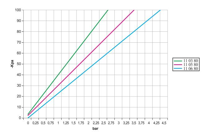
Note: The values shown in the tables are purely indicative as they depend on atmospheric pressure, the flow rate of the vacuum source and the quality of the compressed air supply
